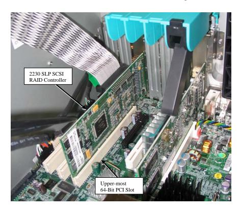
4. Install the N5101A card in the lower 64bit PCI slot. NOTE: Option 022 (2GB DRAM) is required. N5101A PCI cards may vary in appearance.
