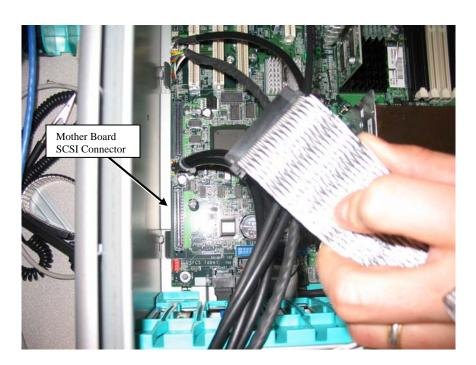
3. Install the Adaptec 2230SLP SCSI RAID controller card in the upper-most 64-bit PCI slot, and attach the SCSI cable removed from step two to the 2230SLP.
